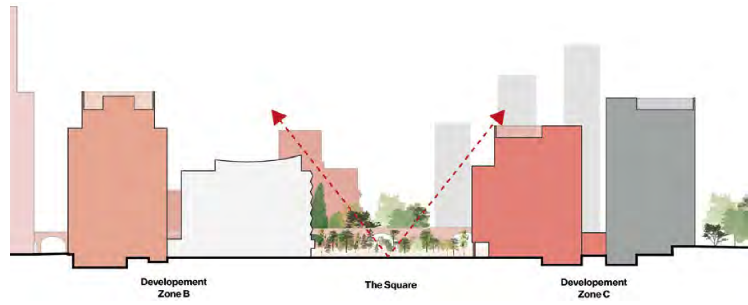
Image: Illustrative site section indicating building heights rising as you move towards to the edges of the Framework Area
